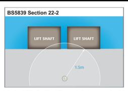
Vertical Shafts like lifts and stairways should have a device mounted within 1.5m of any opening.
