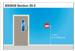
The centre of the frangible element of the manual call point should be positioned 1.4m (+/-200mm) from floor level. (Unless a wheelchair user is likely to be the first person to raise the alarm).
