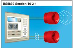
The minimum sound level should be 65dB(A) or Sounder device cabling should be arranged sounder will remain operational during a fire condition.
