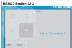
When mounted on a flat ceiling, heat detection devices have an individual coverage of 5.3 radius. However these radii must overlap to ensure there are no 'blind spots'. Therefore individual coverage can be represented by a square measuring 7.5x7.5m giving an actual area coverage of 56.3m2 per device.
