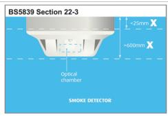
A person searching a zone for a fire in a The sensing element of a smoke detection non-addressable fire system should not have device (optical smoke chamber) should not be to travel more than 60m to identify the source less than 25mm below ceiling, and not greater than 600mm below ceiling.
