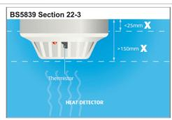
The sensing element of a heat detection device should not be less than 25mm below ceiling, and not greater than 150mm below ceiling.
